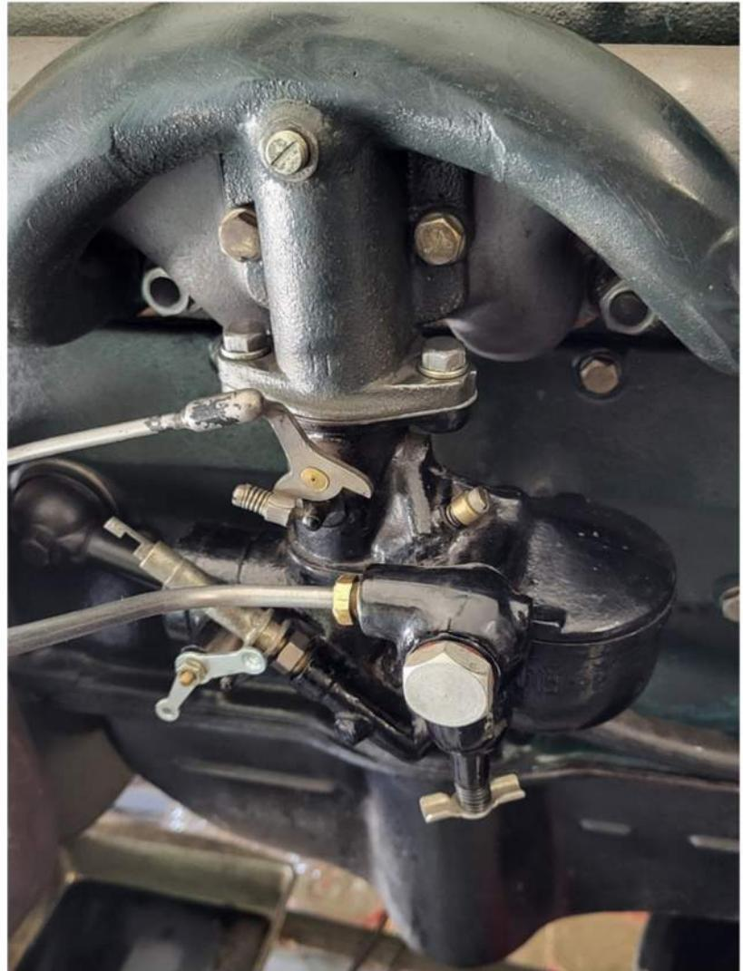
I also heard from Hal that he was going to move his Vicki and found multiple valves were stuck, and Hal said it hasn't been that long since he ran it. Next steps are drop the intake and exhaust manifolds and remove the valve cover to try to free up the stuck valves. Hopefully that works because the next step would be to remove the head and it would be good not to have to go there, right Hal!!
